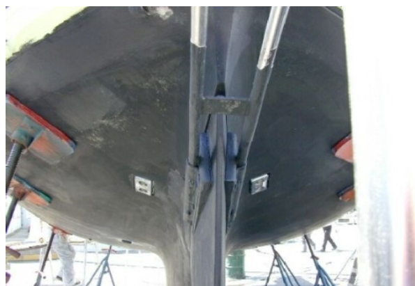
Fairing shims added to the rudder of a Tashiba 40 Pilothouse
